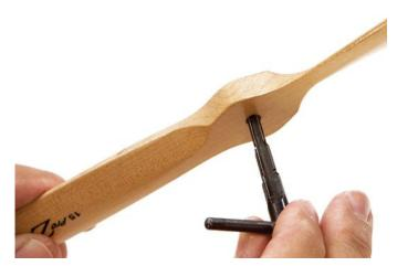
The first step is to enlarge the shaft hole to a size that fits your engine. If you balance the prop first, then enlarge the hole, you will have to come back and balance the prop again, so save some time by balancing afterward. The best way to do this is by using a good prop hand reamer because this will keep the hole concentric.
