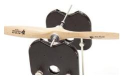
Once the heavy blade is identified and the prop balanced level or within five to 10 degrees in the horizontal plane you can move to the next step.
