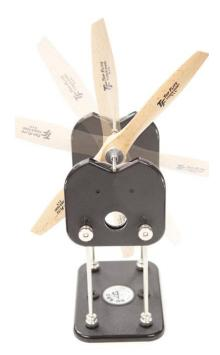
Now move the prop to any position and see if it stays there, if it does then you have a balanced prop. If not keep adjust the amount of CA on the hub by adding or sanding off (in case you over did it) until it does. You may also have to adjust the blade weight to fine-tune the balance.
