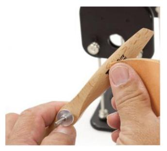
Two methods are commonly used to balance the propeller. The first involves lightening the heavy blade until the propeller balances close to the horizontal position. Use a razor blade or sand paper to remove small amounts of material while rechecking the balance. Don't forget to wipe off any dust or shavings before re-checking the balance.
